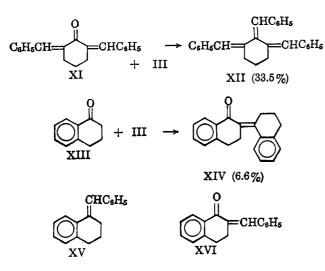
matography and no evidence for its formation was obtained. In addition to the phosphine oxide and recovered XIII, the condensation product (XIV) of XIII was the only material isolated. Attempted reaction of XVI and III led to the recovery of XVI; no evidence for the formation of the expected product, 1,2-dibenzylidenetetralin (XVII), was obtained.
